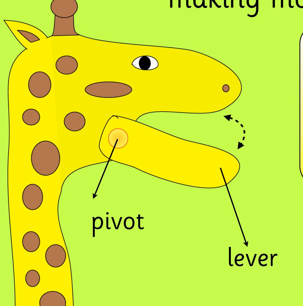
This giraffe has a lever for the bottom part of his mouth which attached to the rest of his face by a pivot. This means his mouth can move up and down.
