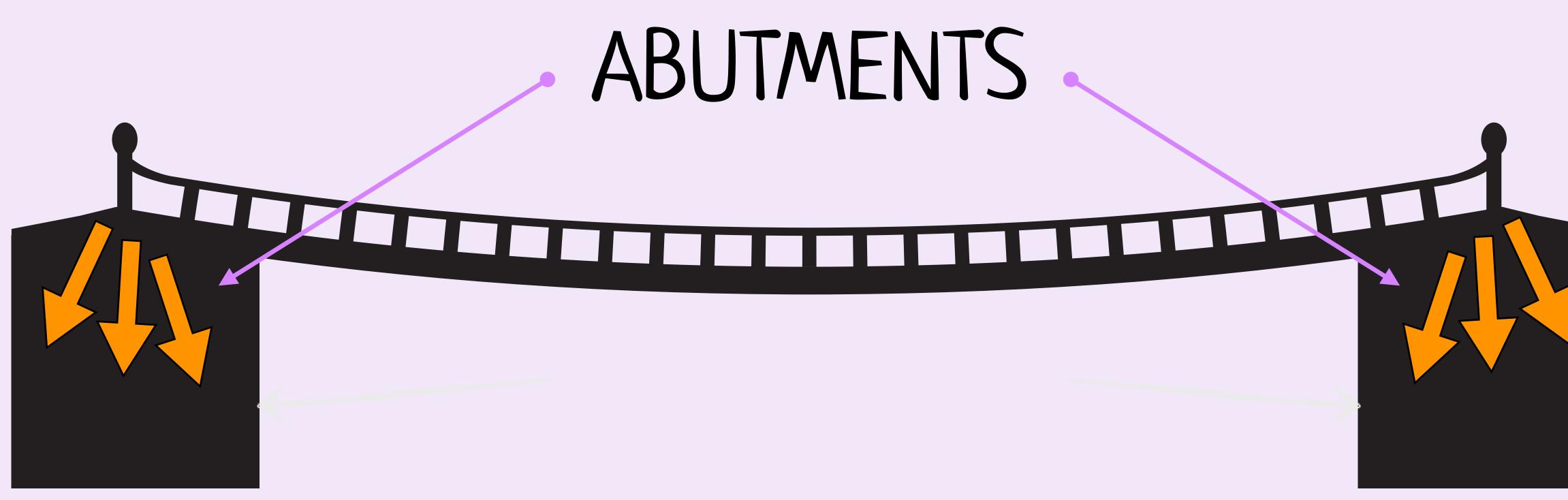
Gravity acts on the beams, decks and pillars of bridges, generating compression forces. The orange arrows show how these compression forces are spread out at either end of the bridge, where it rests on its abutments.
