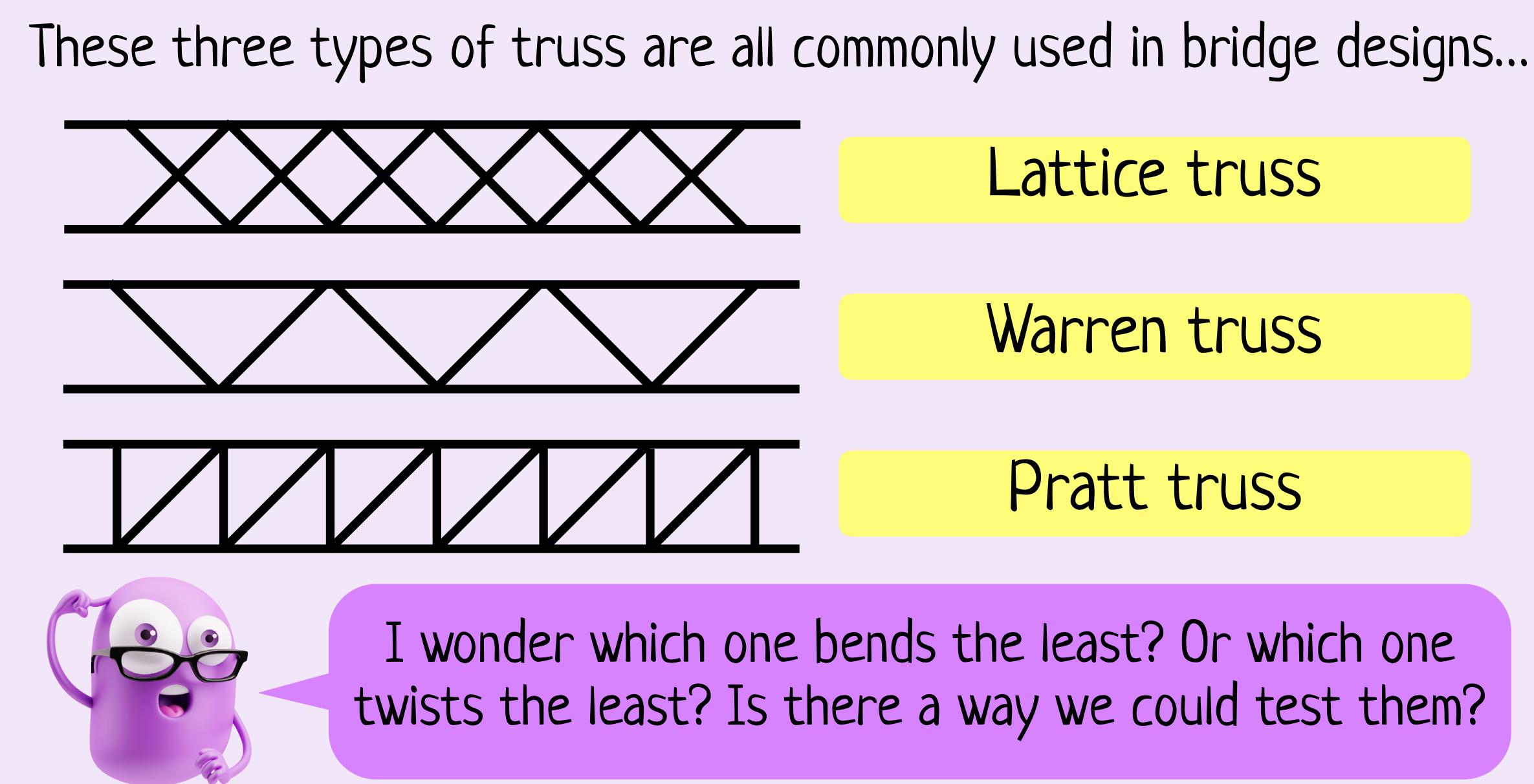
Today we will be exploring ways in which trusses can be constructed and used to strengthen bridges.
